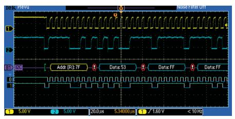
MSO/DPO2000 triggered on a specific data packet going across an I<sup>2</sup>C bus. No more counting clock edges and 1s and 0s. A Bus waveform provides decoded packet content including Start, Address, Read/Write, Data, and Stop. And the addition of timing waveforms makes it easy to quickly determine values of two signals.
